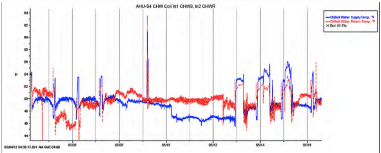
From the chart, it can be seen that throughout the period, the  $\Delta T$  never approached a typical design condition. This is an indication that more water is being pumped through the chilled water coil than is necessary or beneficial.
